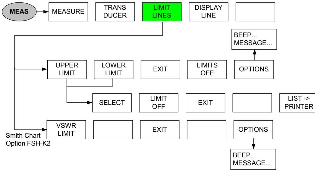
Menus for measurements with isotropic sensor
