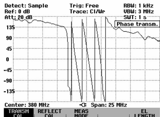
The UNWRAP function removes the restriction limiting the value range to  $\pm 180^\circ$ . With this function, no more shifts will occur, and the phase can have any value from  $0^\circ$  to  $54360^\circ$ . You can activate the UNWRAP function as follows:
