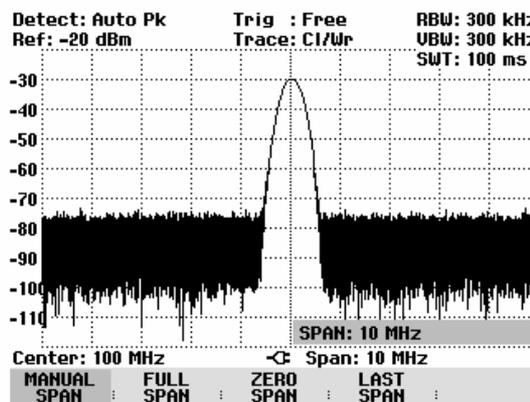
The R&S FSH has markers for reading off signal levels and frequencies. Markers are always positioned on the trace. Both the level and frequency at their current positions are displayed on the screen.
