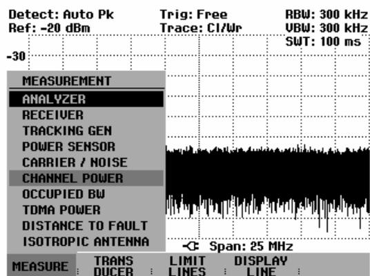
The R&S FSH displays the softkey menu for setting the channel power measurement. Two vertical lines in the measurement diagram indicate the channel bandwidth. The measured channel power is shown in large letters below the measurement diagram.
