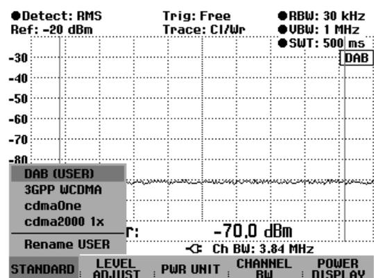
Using the R&S FSH View control software, additional standards can be generated and permanently loaded into the R&S FSH. You can also delete the factory-set standards provided in the instrument if you do not need them. The R&S FSH then offers only the standards you require, for example for measurements on TV signals.
