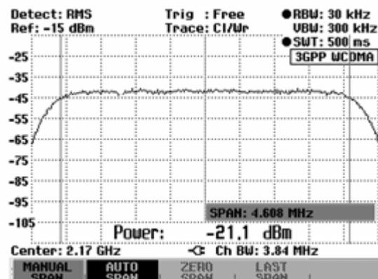
The largest permissible span for the channel power measurement is ten times the channel bandwidth. At larger spans, the result of the channel power measurement would be increasingly imprecise, because too few points of the trace occur in the channel to be measured.
