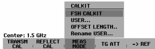
To perform phase correction for additional cables and adapters proceed as follows:
