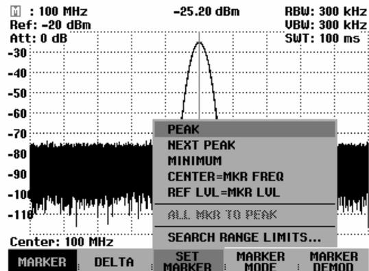
The R&S FSH allows you to use only a limited section of the trace for the PEAK, NEXT PEAK and MINIMUM functions. This is beneficial, for example, if you want to sample only spurious emissions with the marker search functions and want to omit useful signals.
