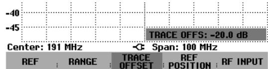
The trace offset function is useful if it is necessary to compensate for a fixed loss or gain during the measurement.
