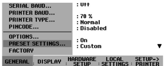
The submenu for selecting the default setup opens. Either DEFAULT or CUSTOM can be selected.
