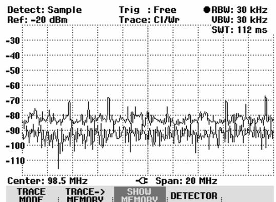
**Note:** The memory trace is bit-mapped into the picture memory. Therefore, when the memory trace is recalled, it will not be adapted to any modifications of the reference level or span that may have been made in the meantime.
