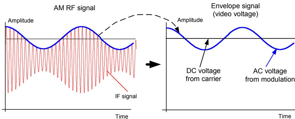
The envelope signal contains a DC component corresponding to the carrier level and an AC component whose frequency is the same as the AM frequency. If the bandwidth of the video filter is less than the frequency of the AC component, the latter will be suppressed depending on its maximum frequency. If the AM component is to be displayed faithfully, the cutoff frequency must be greater than the modulation frequency.
