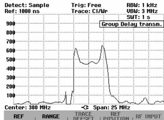
Defining the span for the group delay measurement:
