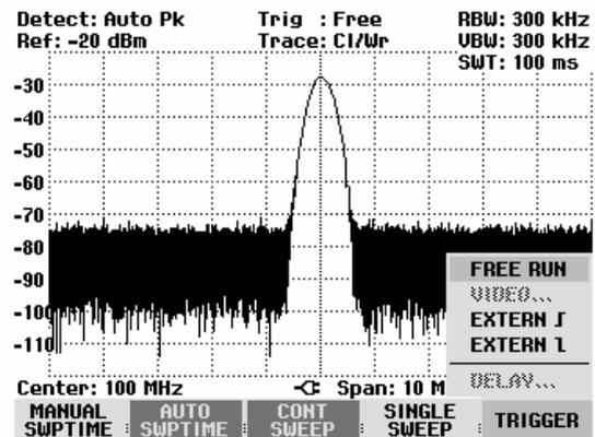
If the VIDEO... trigger setting has been selected, the trigger level and any trigger delay (DELAY...) must be entered. The trigger level is expressed as a percentage (%) of the reference level. 100 % means that the trigger level equals the reference level, 50 % that the trigger level is in the middle of the y axis on the measurement diagram (default setting). The position of the video trigger on the level axis is shown by a ">".
