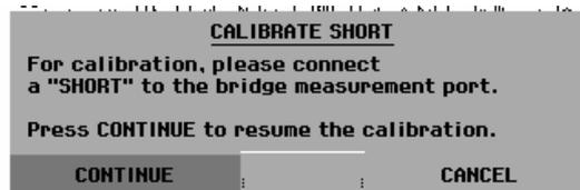
During calibration, the R&S FSH outputs the message "Calibrating SHORT, please wait...". Calibration can be aborted with the CANCEL softkey.
