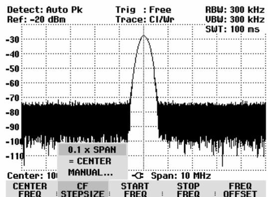
If you select "0.1 x SPAN" or "= CENTER", the R&S FSH makes the setting directly itself. If you select "MANUAL...", the value entry box opens and indicates the current step size.
