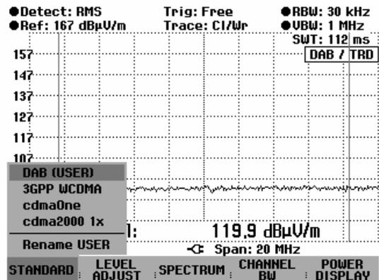
You can also create additional standards by using the R&S FSH View control software and load them into the R&S FSH. You can also use this software to delete factory-supplied standards if you do not need them. The R&S FSH will then offer only the standards you need, e.g. for measuring TV signals.
