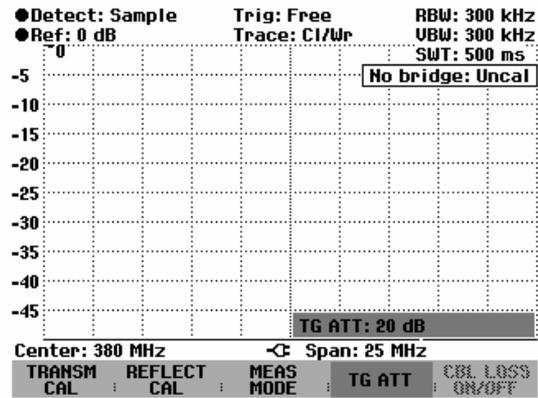
**Setting the tracking generator step attenuator:**
