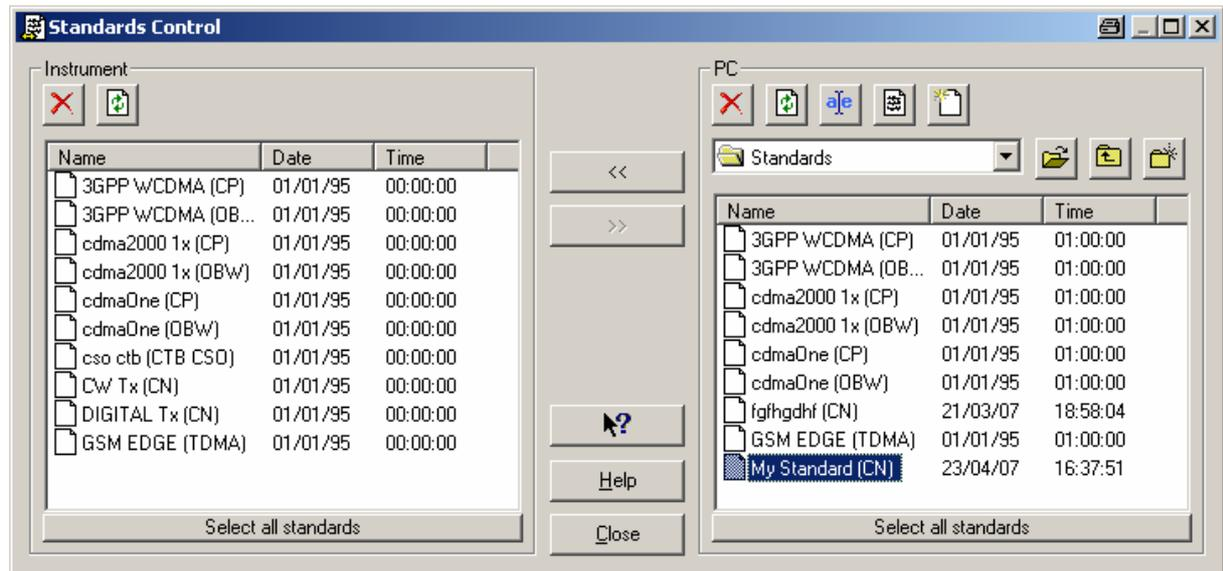
On the left side the standards are listed which are stored in the instrument. On the right side the standards are listed which are stored in the directory ...\\Standards of the PC. Behind the standard name the measurement name is given in brackets. (CN) indicates a carrier / noise measurement standard.
