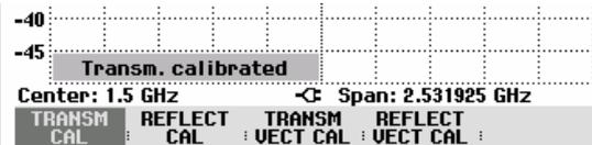
The R&S FSH now displays Transm. in the upper right-hand corner of the measurement diagram. This tells you that the R&S FSH has been calibrated for transfer function measurements. In addition, the TRANSM CAL softkey label is highlighted in green.
