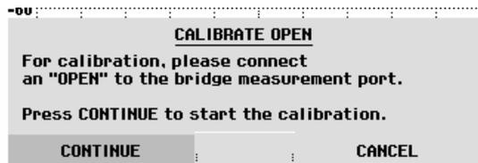
When the open calibration is over, the R&S FSH will prompt you to terminate the measurement port in a short.
