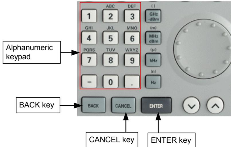
If the R&S FSH is expecting a letter entry, it automatically assigns the letters above the keys to the keys in the alphanumeric keypad. The keys have a multiple assignment. Enter the letter you want by pressing the key in question the appropriate number of times.
