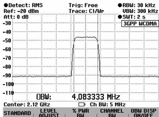
If USER is selected, the R&S FSH restores the last setting used in the USER mode for measuring the occupied bandwidth. The R&S FSH automatically makes changes to the setting so that it is again available when USER is called again.
