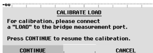
When calibration is over, the R&S FSH outputs the message "Reflect. calibrated" for three seconds.
