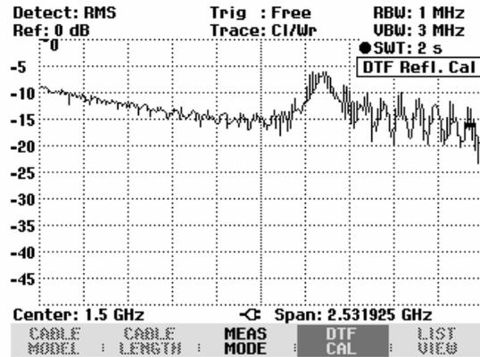
To indicate that the R&S FSH is measuring return loss, DTF refl. cal is displayed in the upper right-hand corner of the screen.
