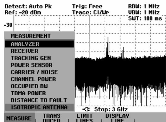
The R&S FSH will open the measurement function menu and activate the Isotropic Antenna measurement function. Before displaying final measurement results, the R&S FSH performs a measurement for each of the three antenna axes so that the update rate of the trace decreases accordingly.
