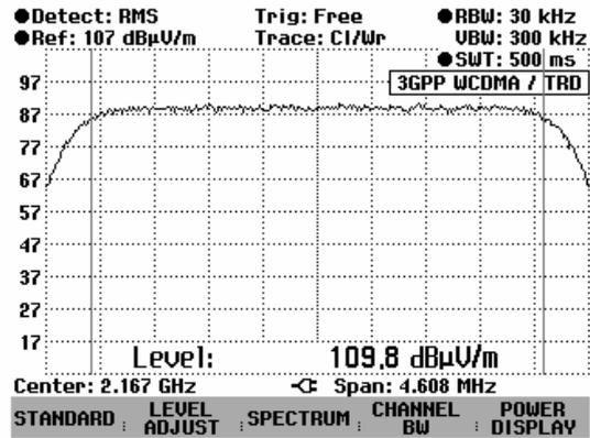
The R&S FSH will display the softkey menu for setting the channel power measurement. It indicates the channel bandwidth in the measurement diagram by means of two vertical lines. It displays the measured resultant field strength in large characters at the bottom of the diagram.
