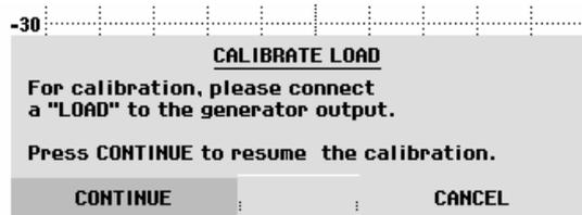
During calibration, the R&S FSH outputs the message "Calibrating LOAD, please wait".
