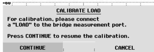
On completion of calibration, depending on the VSWR bridge used, the R&S FSH displays **FSH-Z2: Vector Voltmeter refl.** in the top right of the chart. This indicates that it has been vector calibrated for reflection measurements. Also, the softkey lettering REFLECT CAL has a green background.
