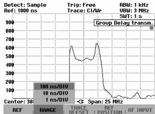
**Transmission measurement using the connected VSWR Bridge R&S FSH-Z3**
