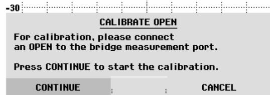
While calibration is in progress, the R&S FSH outputs the message "Calibrating OPEN, please wait...".
