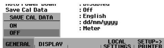
The state for calibration data saving is entered in the SETUP menu.
