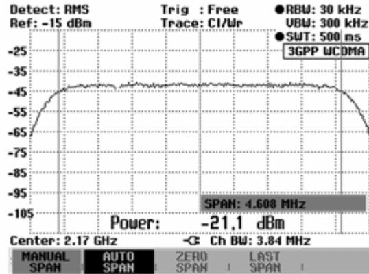
The largest span that is permitted in the channel power measurement is ten times the channel bandwidth. At larger spans, the result would be increasingly inaccurate, because not enough points of the trace are located in the channel to be measured.
