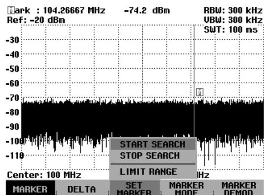
The procedure for entering the stop frequency for the search range is analogous to that for entering the start frequency.
