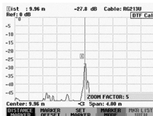
The screenshot on the right shows that the fault of the measured cable consists of two transitions. A coupling of approx. 7 cm in length was used to connect two cables.
