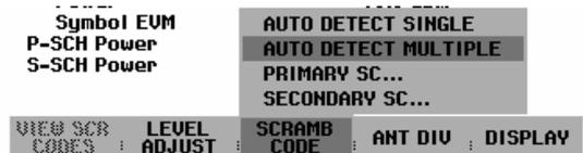
The scrambling code search takes about 50 s. The progress is indicated as a percent figure on the display. As soon as it has found the scrambling codes, the R&S FSH synchronizes to the 3GPP signal with the highest level. The screen will show SYNC OK, and the result values will be displayed.
