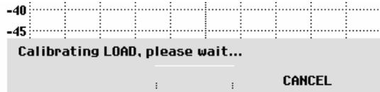
When calibration is over, Magnitude transm. is displayed in the upper right-hand corner to indicate that the R&S FSH is vector-calibrated for transmission measurement. In addition, the TRANSM CAL softkey label is highlighted in green.
