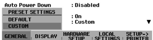
The parameters defined in the data set for the default setup are now used as the preset settings. If no user-specific default setup is defined, CUSTOM is inactive and cannot be selected. The data set defined as the user default setup can be viewed using the R&S FSH's recall function.
