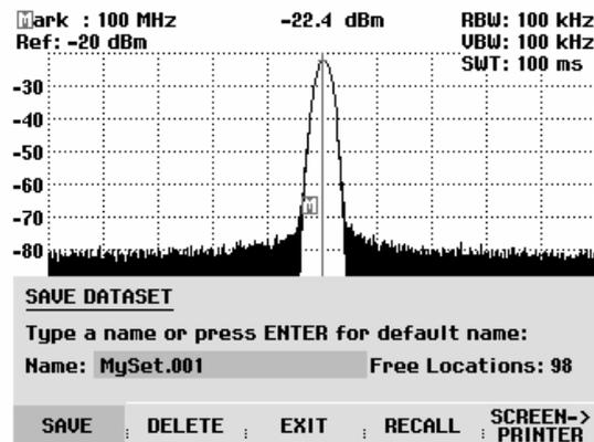
By pressing the BACK key, you can instruct the R&S FSH to browse through the list of names of the data sets already stored and display them with the first available free extension. Thus, the name of the data set recalled for a specific measurement can be selected for storing the measurement data.
