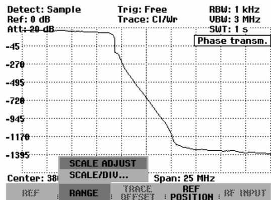
In addition, you can set the y-axis scaling in  $45^\circ/\text{Div}$  increments.
