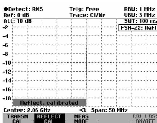
The reflection calibration remains valid until the center frequency or the span is changed on the R&S FSH to such an extent that the new span falls outside the calibrated frequency range. **Uncal** is displayed in the upper right-hand corner of the screen when calibration is no longer valid.
