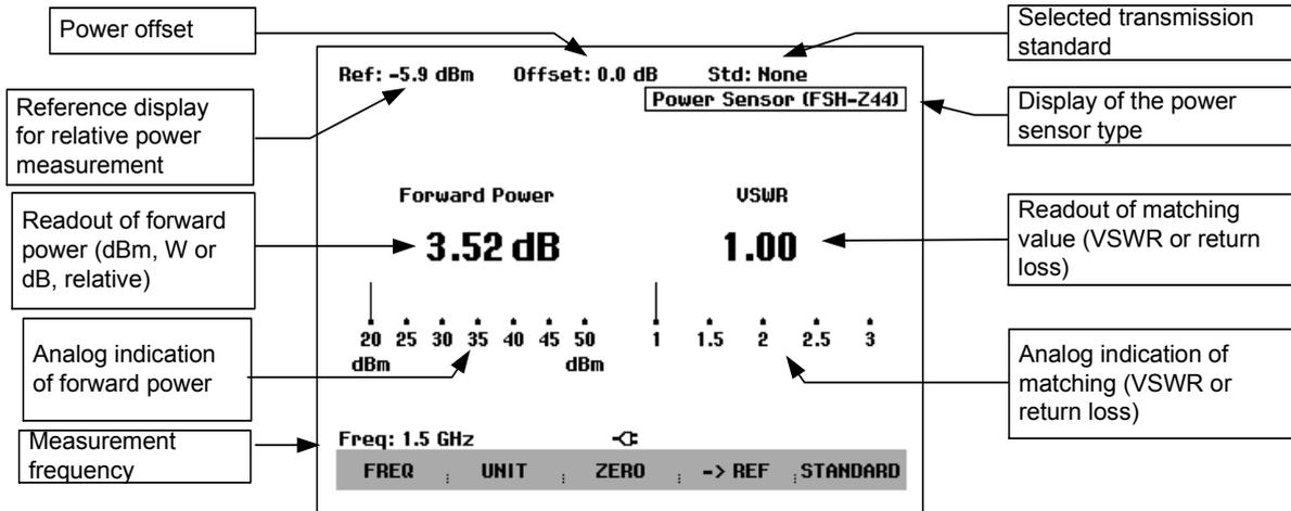
The power sensors contain frequency-dependent correction values. This means that the highest accuracy is reached for signals whose frequency is known. When the R&S FSH switches to the power measurement mode from another operating mode, it transfers its current center frequency to the power sensor.
