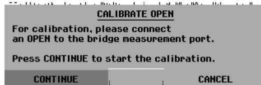
When OPEN calibration is over, the R&S FSH prompts the user to perform SHORT calibration.
