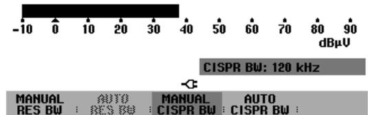
According to CISPR16 the bandwidth is connected to the frequency. The R&S FSH allows to couple the bandwidth to the set frequency automatically:
