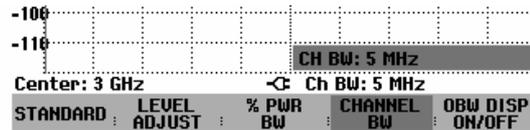
The R&S FSH automatically adapts the span to the channel bandwidth that has been entered (span = 5 x channel bandwidth) to ensure that no incorrect measurements of occupied bandwidth are made. The minimum channel bandwidth that can be set is 2 kHz. If you attempt to enter a smaller channel bandwidth, the R&S FSH will automatically set 2 kHz and output the message "Limit exceeded".
