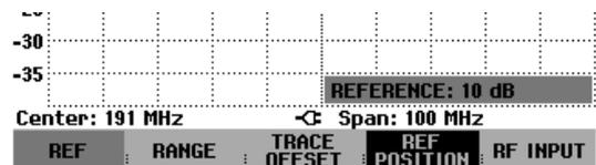
When performing measurements on amplifiers, make sure the R&S FSH is not overdriven. The risk of overdriving is eliminated when the trace is within the display area on the screen (with REF POSITION = 0 dB and TRACE OFFSET = 0 dB).
