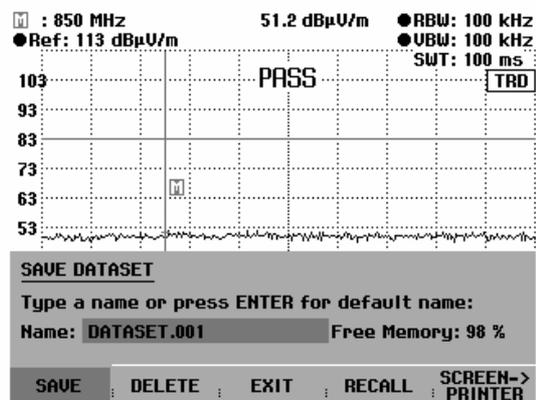
The data set name comprises a text section and a numeric extension, which are separated by a full stop. The data set name suggested by the R&S FSH is derived from the name of the data set last stored, the numeric extension being incremented by 1 in each case.
