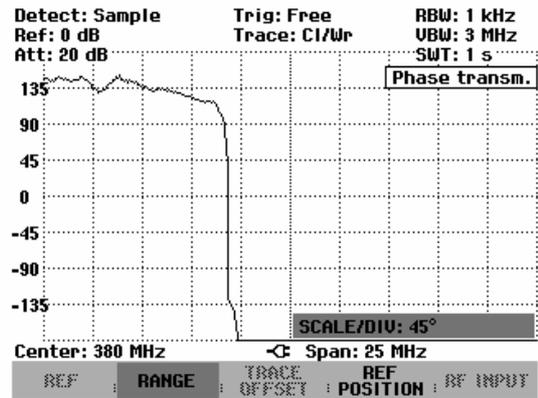
You can shift the reference of the phase measurement, for example to move the test trace to the center of the screen.
