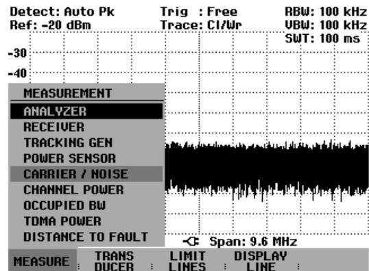
The major measurement parameter settings are available directly in the main menu of the carrier/noise measurement or can be entered using the corresponding function keys.
