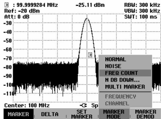
**Measuring the filter bandwidth or the signal bandwidth**
