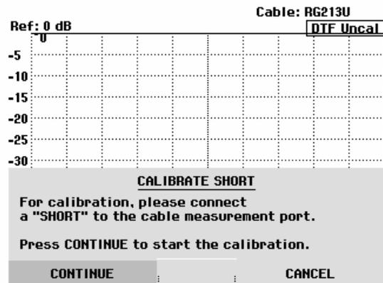
While SHORT calibration is in progress, the R&S FSH outputs the message "Calibrating SHORT, please wait...".
