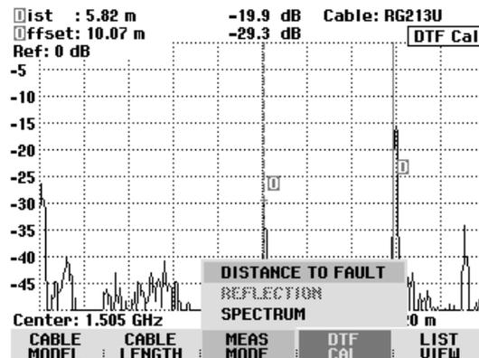
When SPECTRUM is selected, the R&S FSH turns off the tracking generator and displays the spectrum over the frequency range of the DTF measurement. To indicate that the R&S FSH is in the spectrum mode, DTF Spectrum is displayed in the upper right-hand corner of the screen. Otherwise, the R&S FSH uses exactly the same settings as it did for DTF measurements.
