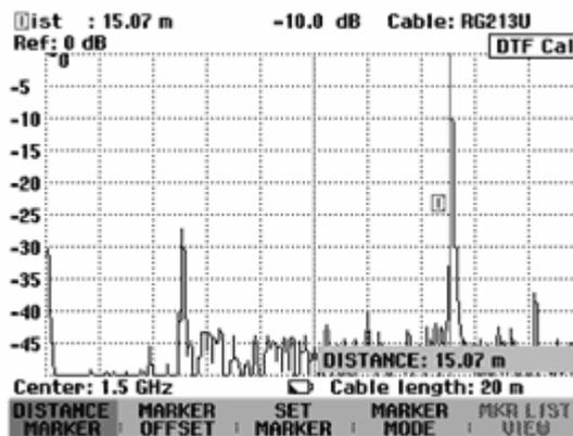
For higher fault resolution, the R&S FSH offers a zoom function in the position of the marker. The x axis of the display can be extended up to a span of 3 m.
