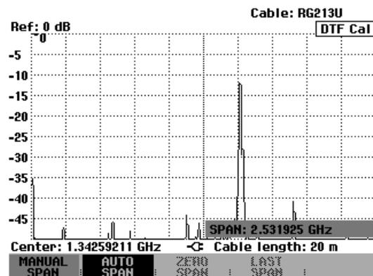
The minimum span that can be set is either 1/10 of the span automatically set by the R&S FSH in the case of AUTO SPAN or 200 MHz (whichever is smaller). Spans larger than the ones set by the R&S FSH with AUTO SPAN are not allowed. If an attempt is made to set smaller or larger spans, the R&S FSH responds with "Minimum reached" or "Range exceeded".
