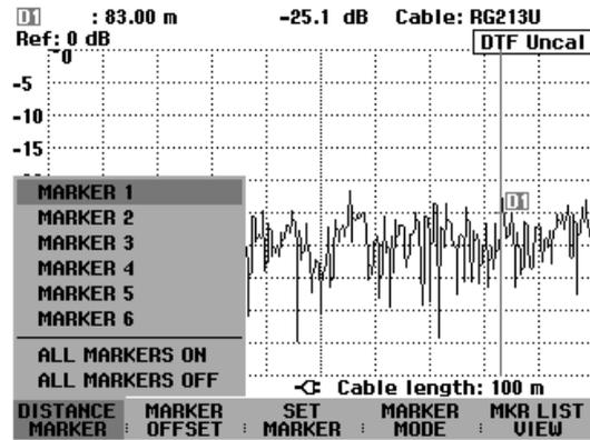
After a marker is activated, its position is indicated in the value entry box. To vary the marker position, use the number keys to enter a distance (e.g. 11.5 m), or move the marker pixel by pixel with the rotary knob, or move it in steps of 10% of the displayed cable length by means of the cursor keys. For fast marker positioning, it is recommended that first coarse adjustment be performed with the cursor keys, and then fine adjustment with the rotary knob.
