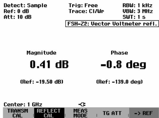
The saved reference values are displayed on the screen below the relative values (in this case **Ref: -19.50 dB and Ref:-139.0 deg** ).
