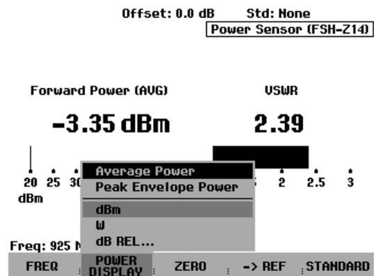
When the dB REL... unit is selected, an entry box for the reference level opens.
