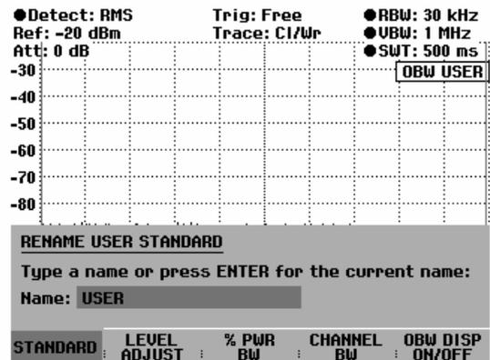
When the STANDARD menu is called, the entered name appears under USER (e.g. DAB (USER)). The name also appears at the upper right-hand corner of the screen after the USER standard is selected.
