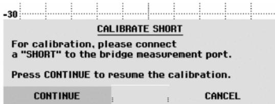
When calibration is over, the R&S FSH outputs the message "Reflect. calibrated" for 3 seconds.
