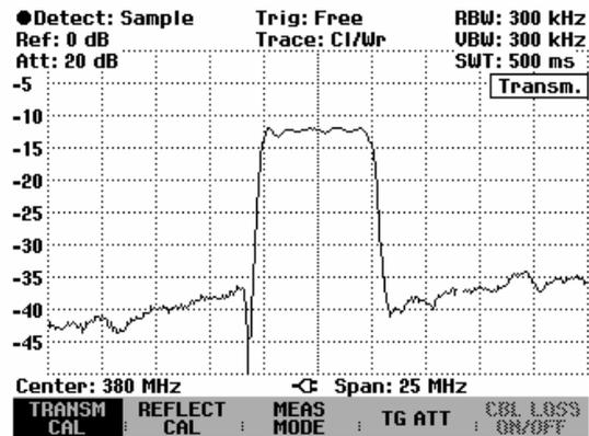
The transmission calibration remains valid until the center frequency or the span is changed on the R&S FSH to such an extent that the new span falls outside the calibrated frequency range. Uncal is displayed in the upper right-hand corner of the screen when calibration is no longer valid.
