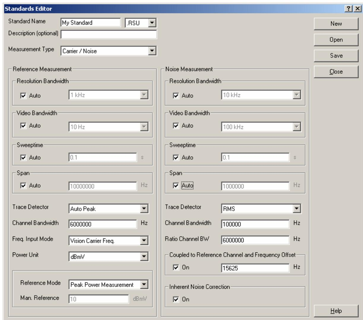
The standard settings are stored in the PC and can be transferred and stored to the instrument R&S FSH via the PC cable.
