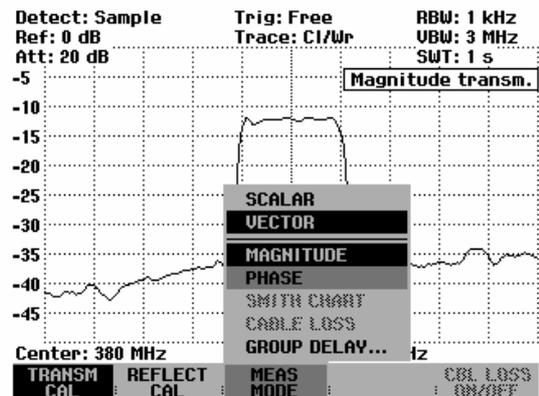
The R&S FSH displays the DUT's phase characteristic as a function of the frequency. Phase transm. will appear in the upper right-hand corner of the display. In the default scaling, the phase can only have values between  $-180^\circ$  and  $+180^\circ$ .
