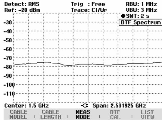
The spectrum mode is used to check if there are any spurious signals in the frequency range of the DTF measurement. These are most likely to be present if the cable under test is connected to an antenna.
