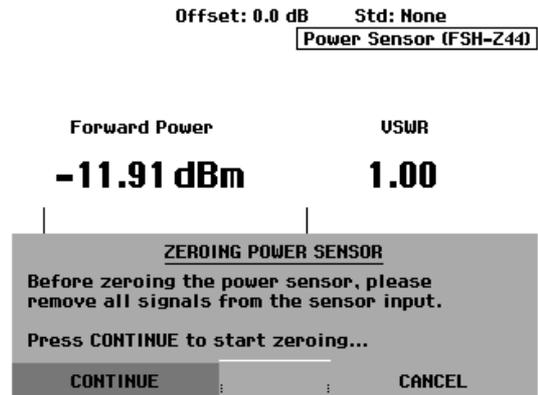
The R&S FSH immediately starts power sensor zeroing. While this is being done, the R&S FSH outputs the message "Zeroing power sensor, please wait...".
