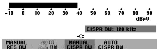
The bandwidths 200 Hz, 9 kHz, 120 kHz and 1 MHz are available.
