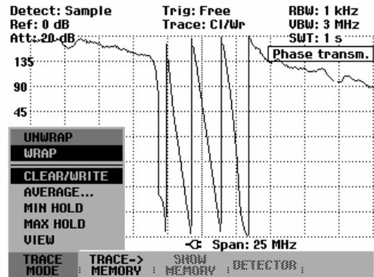
The R&S FSH will now show the phase characteristic without the value range being restricted to  $\pm 180^\circ$ .
