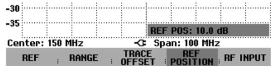
In addition, the trace can be offset without changing the reference and the scale of the y axis.
