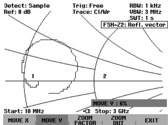
**Measuring the group delay when measuring reflection**
