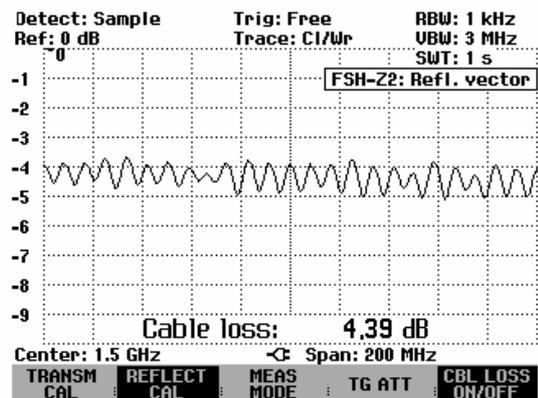
The R&S FSH calculates the cable loss from the average of the maximum and minimum values of the displayed trace. Thus, the cable loss is an average value within the displayed frequency range. Loss at specific frequencies can be determined with one or more markers.
