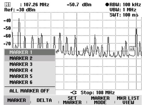
The R&S FSH opens the entry box for the frequency of the selected marker or the spacing between the delta marker and the reference marker M1.
