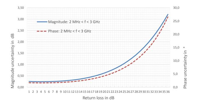
Uncertainty of reflection measurements with the R&S®ZN-Z103 calibration unit; temperature: +18 °C to +25 °C, RBW: 10 Hz, power: -10 dBm.
